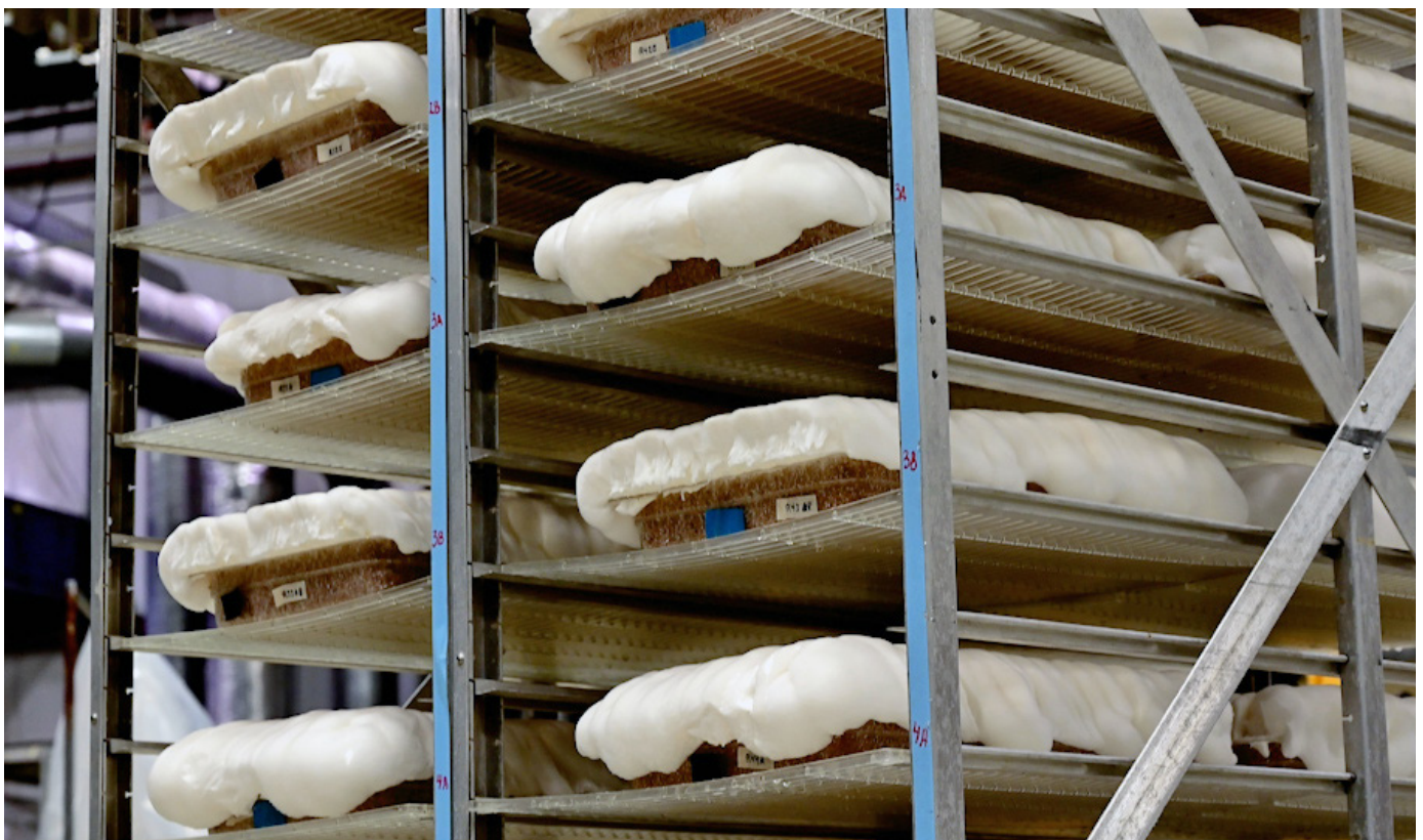
Ecovative grows sheets of mycelium in shelves in its vertical farm. The mycelium, which is propagated from small cuttings of mushrooms, feeds on agricultural waste in special incubation conditions. Ecovative.
